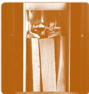
Now ignite the lighting aid and close and lock the door. Make sure that the lock engages properly. The wood burns from top to bottom.
